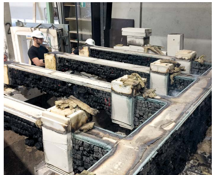
^ All SHERPA connections have withstood a fire exposure of over 90 minutes
