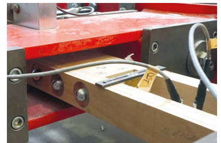
^ Tension plate joint: Experimental determination of the performance potential
