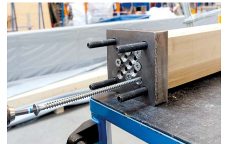
^ Screw group set in end-grain of beech glulam: compact connections with high efficiency
