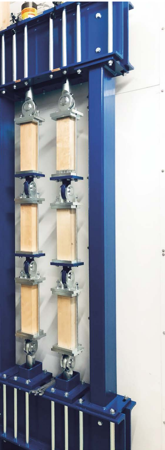
< Testing framework for long-term tests at the Technical University
