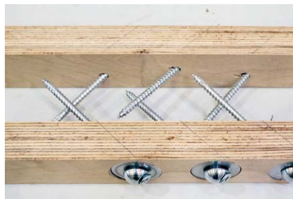
^ Tension plate joint: external plates made of laminated beech veneer including screw arrangement
