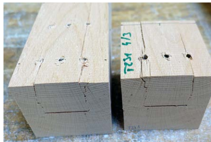
^ Typical cracking: Failure pattern during block shearing of axially stressed screw assemblies
