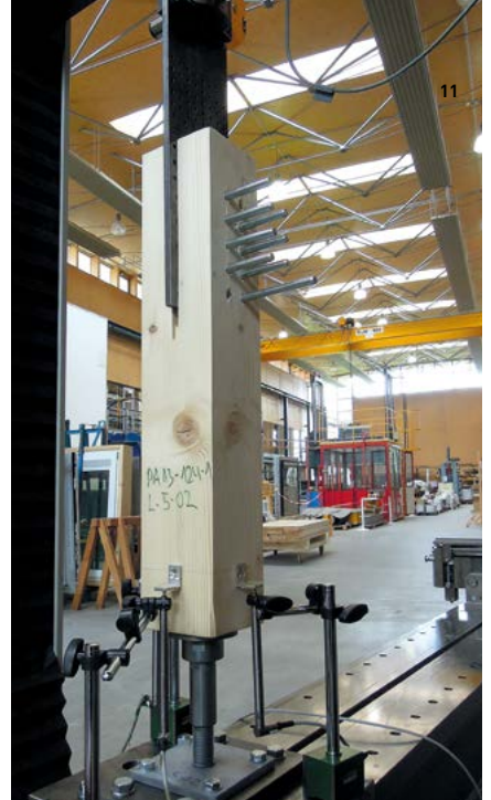
^ Centric tension load: This test was able to demonstrate the performance of the spatial bolting in the case of lifting forces due to wind suction loads, for example.
