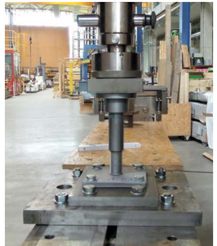
^ Centric load on compression without wood cross-section: This test was an all-steel configuration, where the maximum pressure bearing capacity of the Power Base was determined.
