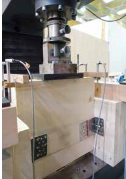
^ Figure 2: Testing the Sonus at the ceiling-wall joint with stress in direction 2/3
