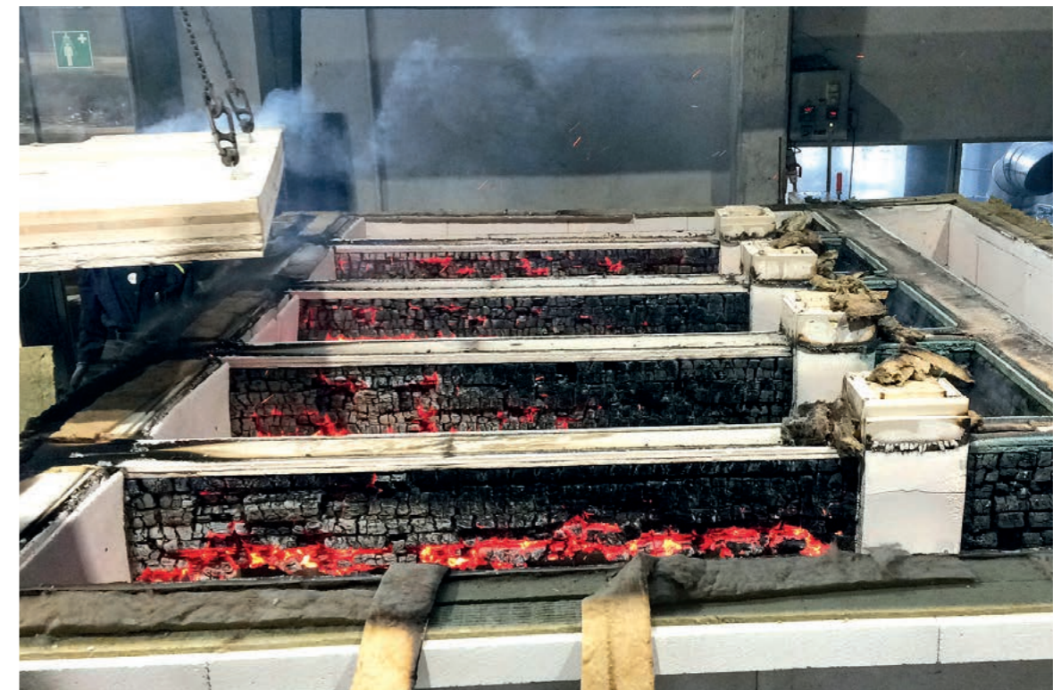
^ SHERPA Fire Test: After the test time expired, the furnace chamber was quickly opened and extinguished.
