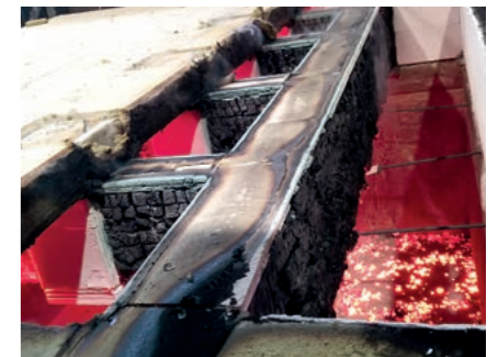
^ SHERPA test bench: A total of 4 loading test specimens for R90 and R120 were tested and the deformations were measured.
