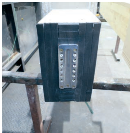
^ SHERPA Fire Stop 2.5: The fire protection laminate protects the connector from direct exposure to temperature in case of fire.
